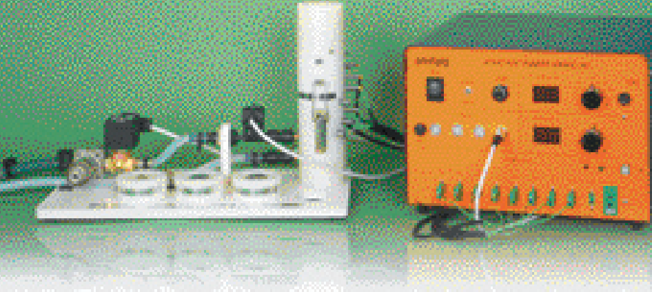
• HT10XC Heat Transfer Service Unit Shown with one of the available accessories, the HT11C Computer Controlled Linear Heat Conduction unit
